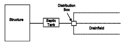
2. Septic tank, drop boxes, drainfield \* generally used on sloping ground
