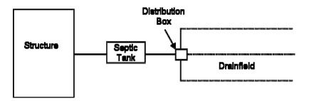
Septic tank, drop boxes, drainfield generally used on sloping ground
